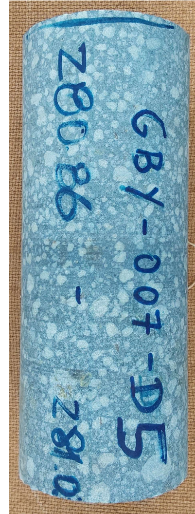
Megacrystic andesite (late-post mineralization) GBY007 280m
