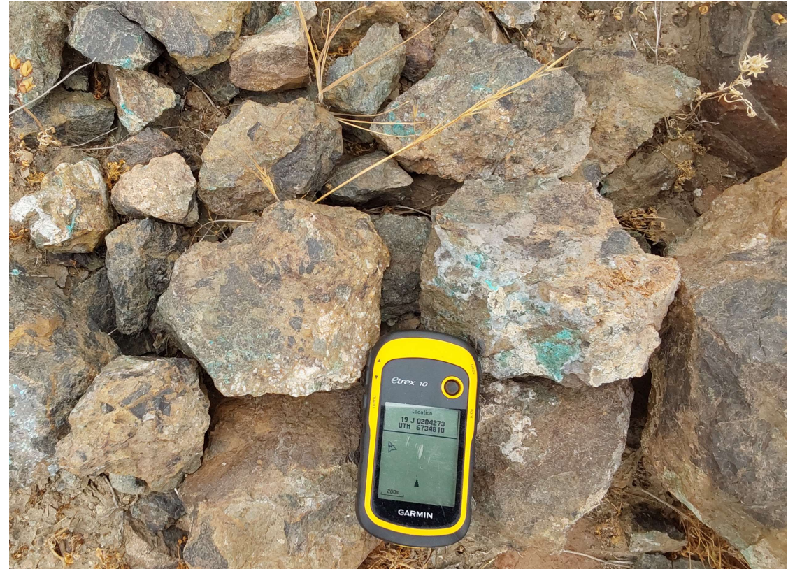
Copper oxide visible with ferruginous material in small pit
